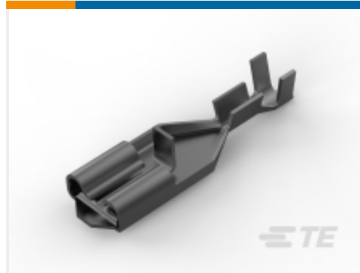
TE Part # 170327-1 250 PL MKII REC. 22-18AWG PTBR
